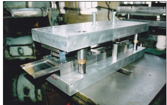
Multi-stage press tool for the lighting industry
